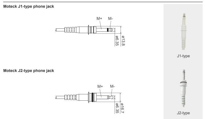
Note: Connect (M+) to '+' & (M-) to '-' of DC power, the actuator will extend.
