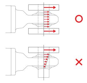
(7) If the actuator is used on the equipment to rotate with the mounting pin as the axis, it must be ensured the housing and other mechanical parts will not interfere and damage the actuator or equipment in the full range of movement.
