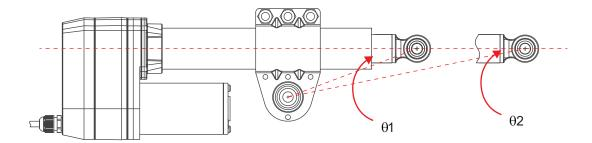
(5) Make sure all the mounting holes of front connector and clamp are at the right position, then lock all the screws, and then confirm all of them are tightened properly.
