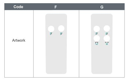
Button definition: Artwork codeF, G 1) Actuator#1 extends 2) Actuator#1 retracts ③Actuator#2 retracts
