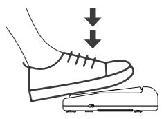
3. By releasing the pedal and allowing it to spring back, the internal safety mechanism will return to its original position and the pedal function will return to normal and be available for use.
