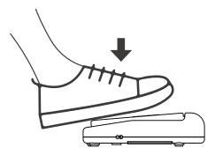
2. If additional force is applied to the down pedal and the pedal is pressed deeper, whether intentionally or unintentionally, an internal safety mechanism (optional) releases the switch and immediately stops the descent.
