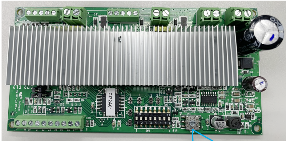
Over-current protection setting
