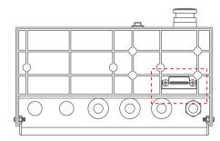
Loosen the screws and remove the cover by sliding it aside.
